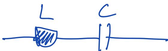
$$\underline{Z}_{\text{eq}} = j \left( \omega L - \frac{1}{\omega C} \right)$$
