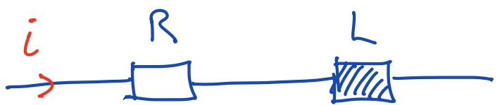
$$U_R = 100 \text{ V} \quad U_L = 100 \text{ V}$$
