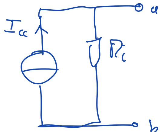
$$I_{cc} = I_{ab} \quad \left| \begin{array}{l} (\text{en courant}) \\ U_{ab} = 0 \end{array} \right.$$
