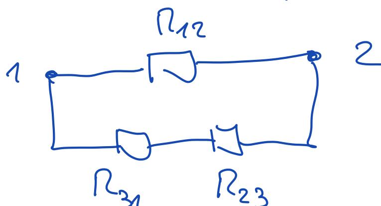
$$R_{eq} = \frac{R_{12} \cdot (R_{31} + R_{23})}{R_{12} + R_{31} + R_{23}}$$
