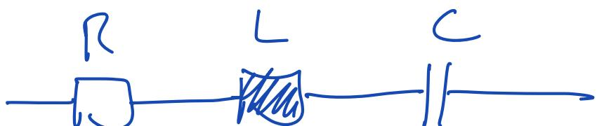
$$\underline{Z}_{\text{tot}} = R + j \left( \omega L - \frac{1}{\omega C} \right)$$
