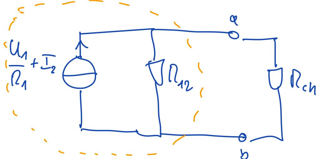
$$R_{12} = \frac{R_1 \cdot R_2}{R_1 + R_2}$$
