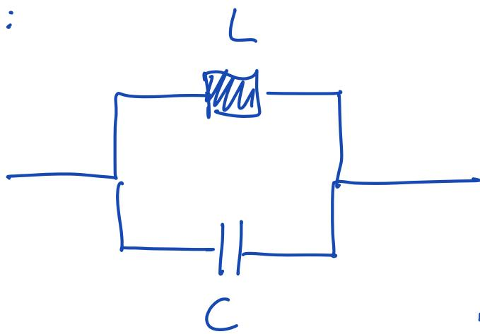
$$\underline{Z}_{eq} = \frac{1}{\frac{1}{j\omega C} + j\omega L} = \frac{j\omega L}{1 - \omega^2 LC}$$
